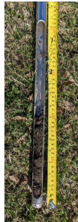
Figure 2. Mark probes at the desired depth to maintain consistent sampling.
